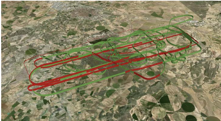
Figure 10: (SKR012) - Flight Trajectory: red represents pilot in control, green closed loop flight
